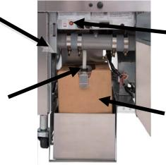
**D: Top off reset button:** Press and hold orange button after replacing the oil until top off empty notice goes out.
