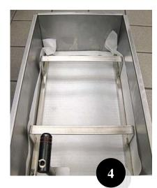
The filter pan must be cleaned daily and the filter paper replaced. Follow these instructions to prepare the filter pan:
